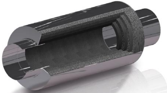
03 ALANTUM silencer with absorber consisting of several layers of heat- and corrosion-resistant alloy foam
