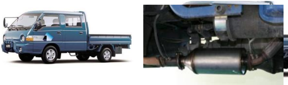
Figure 9: Light duty diesel truck and installed ALANTUM foam filter
